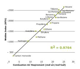
The table and graph above show the relationship of Wobbe Index and the Stochiometric Dry Air Requirement for some typical gas constituents. The correlation is close to linear ( $R^2 = 0.9764$ ) with an intercept close to zero. The residual oxygen method takes advantage of this correlation by linear extrapolation between measurements of known calibration gases.  $R^2$  for typical natural gas constituents plus hydrogen and CO is 0.9888.
