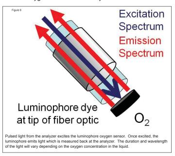
The Barben luminophore sensor is specifically designed for use in industrial applications such as SAGD water treatment. The sensor is unaffected by poisons such as H<sub>2</sub>S or other chemicals that often damage traditional electrochemical sensors. The sensor uses no membrane thus cannot be fouled by particulates or oils. Calibration intervals are much longer than electrochemical cells with 3-6 months as typical.
