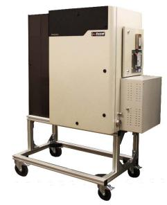
**Figure 5.** The MAX300-RTG, real-time mass spectrometer. For refinery flare compliance, the analyzer is often configured with a Hazardous Area Certification and corrosive-resistant materials that perform well with highlevel H<sub>2</sub>S and HF acid, according to site requirements.
