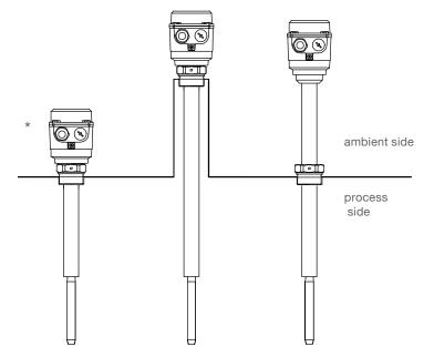
\* Max ambient temperature is derated when process temperature exceeds 60°C (140°F), see (1) on page 7.
