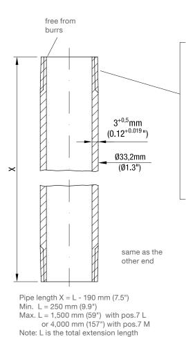
\*Version with R 1" thread Thread R 1" EN 10226 Effective thread length: 14.5 .. 19.1 mm (0.57 .. 0.75") (dimension L1 according to standard EN 10226)
