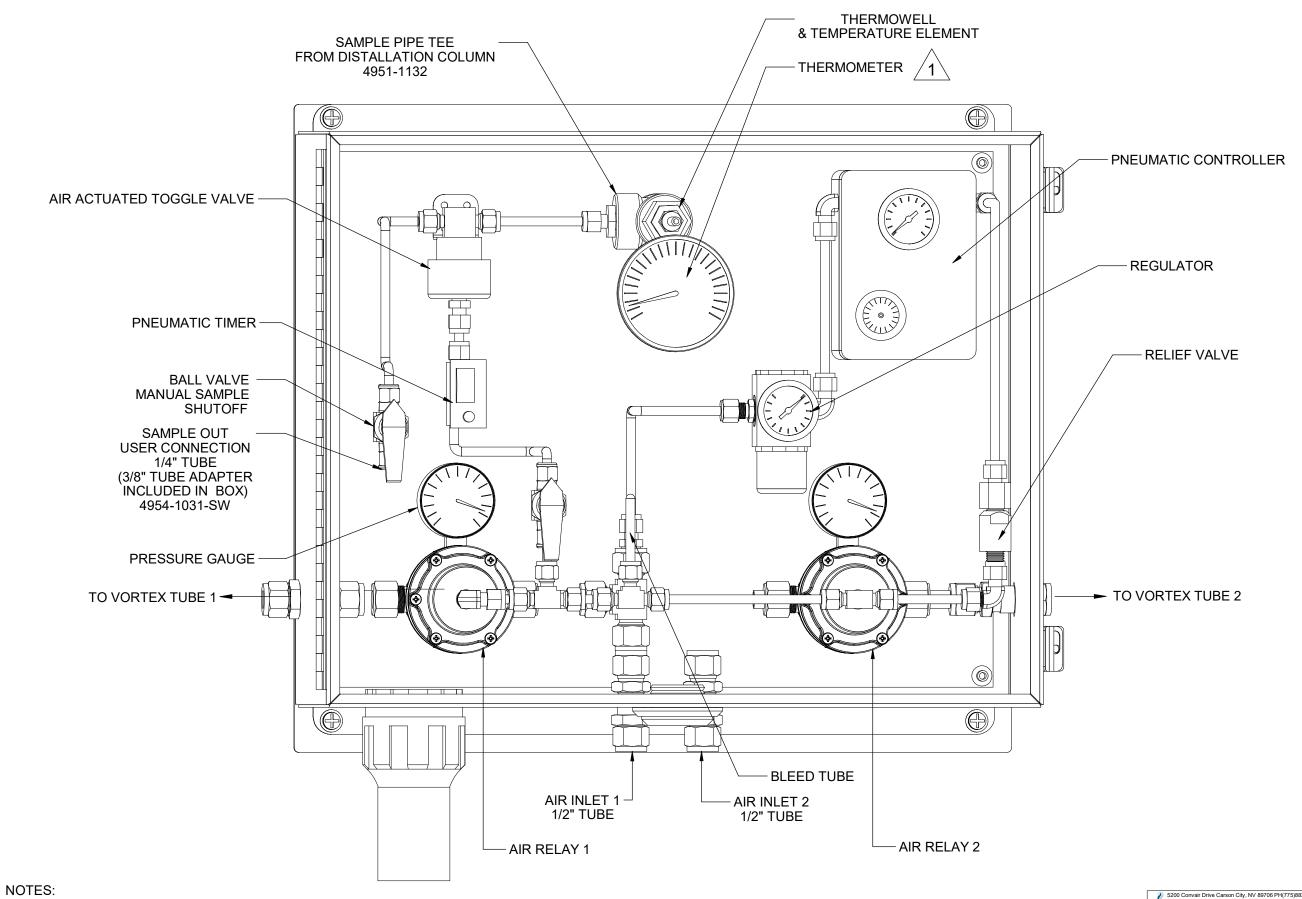
1 THE THERMOMETER EXTENDS INTO THE MAIN COLUMN AND MUST BE REMOVED PRIOR TO REMOVING THE DISC ASSEMBLY. THERMOMETER TO BE INSTALLED UTILIZING A BORED-THRU COMPRESSION FITTING FOR EASE OF REMOVAL AND PROPER SEAL.
